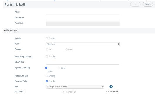
Figure 3 Network Port Configuration
